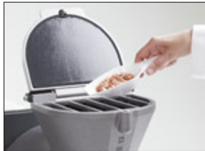
Comminution of ceramic with the Disk Mill PULVERISETTE 13 premium line – gap width 0.7 mm
