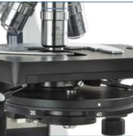
Zernike phase contrast condenser with filter holder
